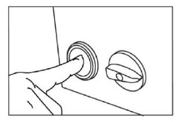
**CAUTION:** Make sure the intervals between pressing the switch are longer than 10 seconds. The engine electric start motor requires 10 seconds to cool between uses. This will also help extend the battery life.
