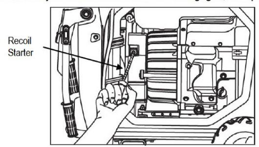
Note: Grasp the generator handle firmly to prevent the generator from falling over when pulling the recoil starter.
