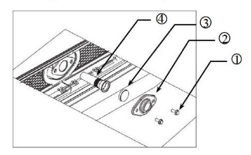
b) Remove spark arrester bracket②, flame screen③, and spark arrester④.
