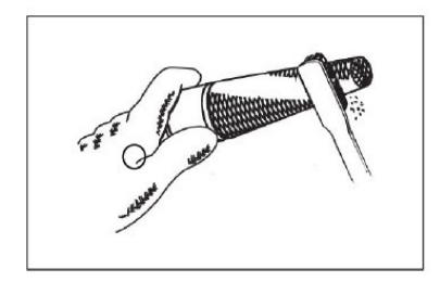
NOTICE: When cleaning, use a wire brush lightly to avoid damaging or scratching muffler screen and spark arrester.
