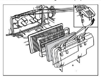
d) Replace paper filter with a new filter.
