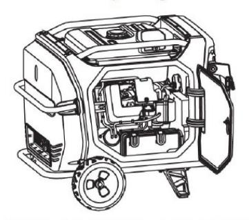
c) Remove the air filter housing cover, paper filter, and foam element.
