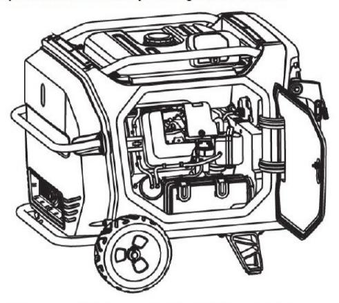
b) Remove spark plug cap③. Insert the spark plug wrench onto the spark plug and turn it counter clockwise to remove the spark plug.
