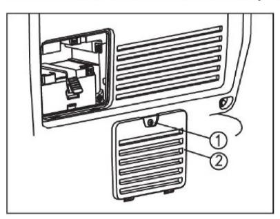
b) Open the fuse cover③. Replace any bad fuses with the same rated fuse.
